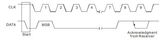
The audio processor that has been addressed has to generate an Acknowledge after receiving each byte, otherwise, the SDA Line will remain at the High Level during the ninth (9th) Clock Pulse. In this case, the master transmitter can generate the STOP Information in order to abort the transfer.
