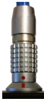
Figure 10 - Lemo Connector to GK-404
