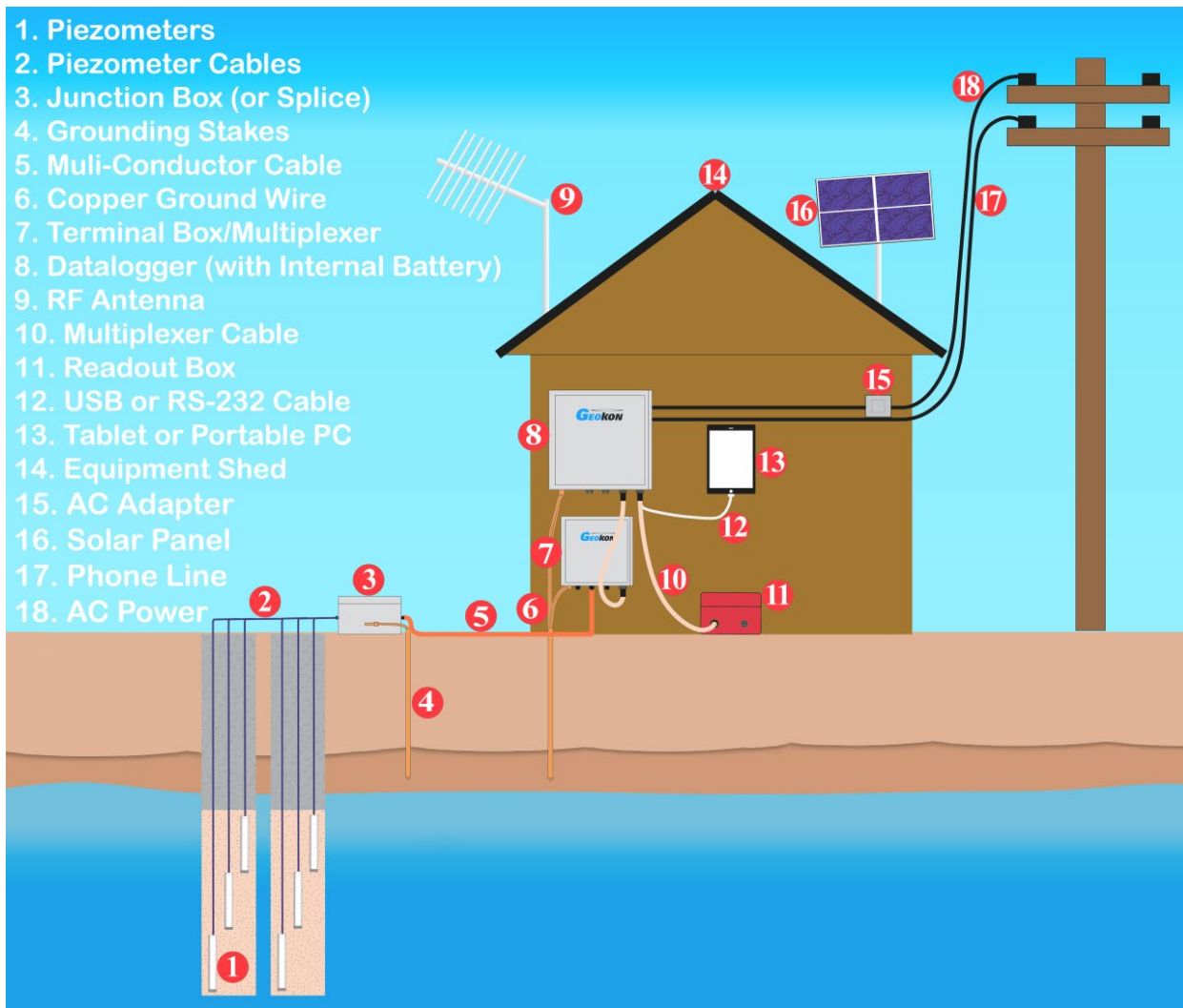
Figure 8 - Typical Multi-Piezometer Installation
