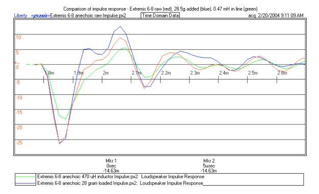
You can clearly see that the raw and mass loaded transient peaks - first negative and first positive peaks - occur at the same time. The inductively loaded (green) peaks are definitely delayed in time. As one would expect!
