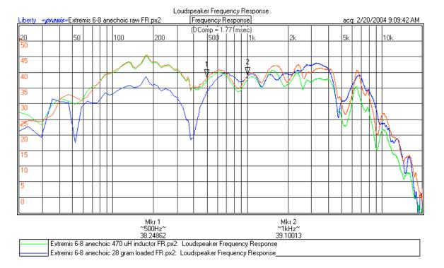
Note the red and blue - raw and mass loaded, respectively. They are pretty much equal from 700 Hz and up (I assume we all accept the Fourier transforms, and that the Fs/efficiency of the driver is affected by the added mass, accounting for the differences down low.
