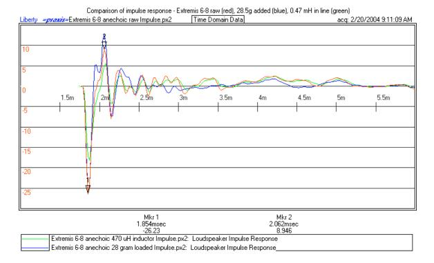
Raw image dump from Praxis. Red is the raw driver - nothing added. Blue is the driver with 28.5 grams mass added. Green is the driver (no added mass) with the inductor in series.
