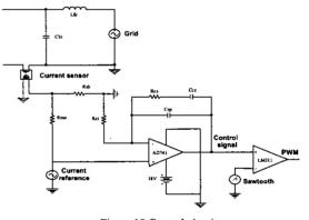
Figure 10 Control circuit
