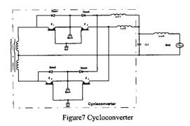
The two bi-directional switches work with a small conduction time overlap to make sure that always there will be a path for the inductor current to flow.
