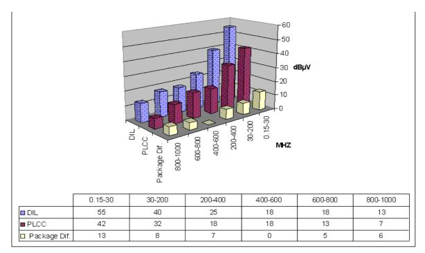
Figure 23. Package effect on the radiated emissions
