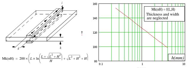
Figure 7. Mutual inductance versus the length and the height of PCB traces
