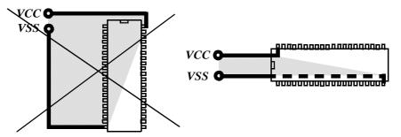
Figure 8. The surface of the VCC and VSS network has to be reduced
