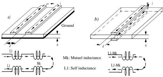
Figure 5. Structure of a parasitic inductance
