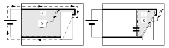
Figure 4. Decoupling capacitor reduces the magnetic field and the loop surface.
