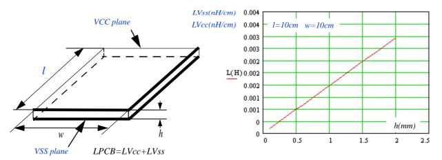
Figure 17. Power-supply planes characteristics
