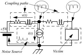
Figure 1. Elements of EMC environment
