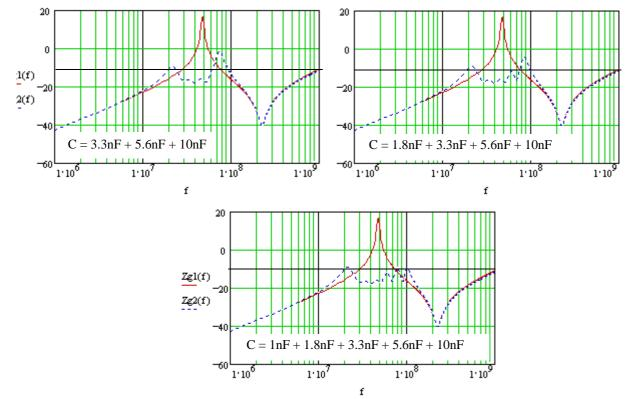
Figure 20. Decoupling effects on the network
