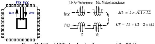
Figure 11. VSS and VCC pins close together can cancel the Hfield
