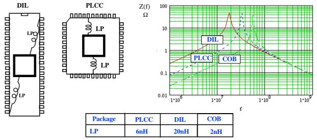
Figure 22. Impedance for a DIL, PLCC and a COB.
