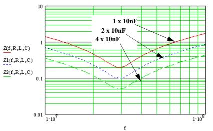
Figure 24. ESR is reduced by connected severals identicals capacitors in parallel
