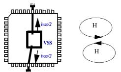
Figure 12. Double and opposited VSS pins reduce 3 to 4dB the H field
