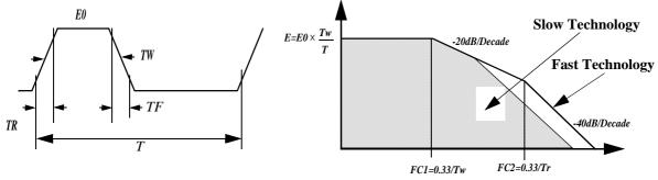
Figure 2. Spectrum of the trapezoïdal signal for a fast and slow technlogy
