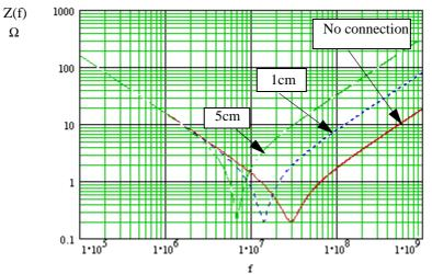
Figure 21. Connecxion increase the impedance in H.F
