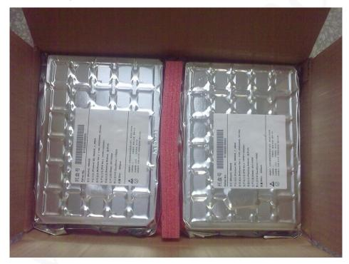
Neoway adopts trays to hold our modules to facilitate mounting. You can just put the tray in fixed direction on your machine. For more details about the storage and mounting of our modules, refer to *Reflow Soldering Guide for Neoway SMD Modules V1.2*.
