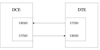
The UART of M590E V1 works at **2.8 V** CMOS logic level. The voltages for input high level should **not** exceed 3.1 V. Supported baud rates are 9600, 14400, 19200, 38400, 57600, 115200 bit/s, and the default rate is **115200 bit/s**.
