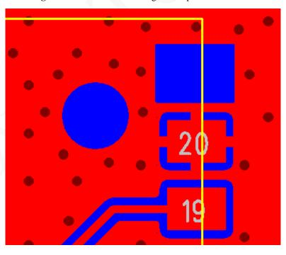
Figure 3-20 Reference RF design when pin 21 is not used
