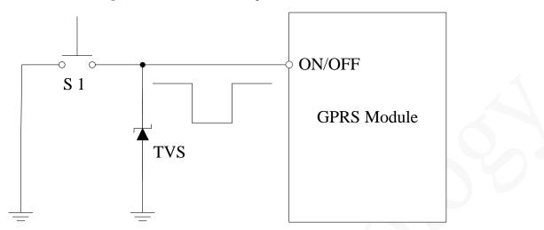
Figure 3-8 Reference circuit for power-on/off control
