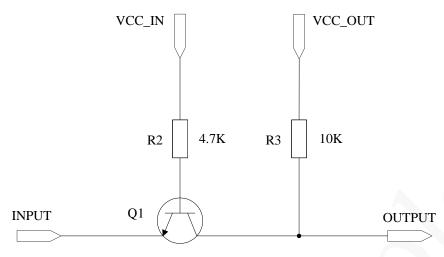
In Figure 3-13, INPUT is connected to UTXD of the MCU and VCC\_IN is connected to the 5 V power supply of the MCU. OUTPUT is connected to URXD of the module and VCC\_OUT is connected to VDD\_EXT(2.8V) of the module. If the circuit is far away from the VDD\_EXT pin, add a 0.1  $\mu$ F decoupling capacitor to VCC\_OUT.
