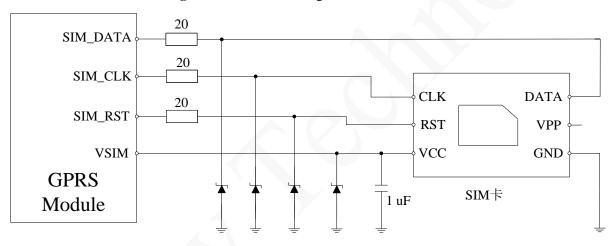
Figure 3-14 Reference design of SIM card interface
