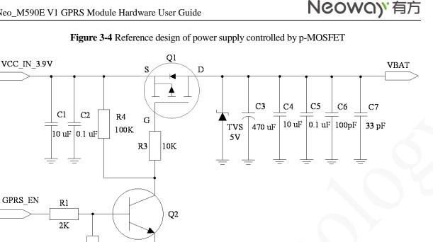
Q2 is added to eliminate the need for a high enough voltage level of the host GPIO. In case that the GPIO can output a high voltage greater than VCC\_IN\_3.9V - |V<sub>GS(th)</sub>|, where V<sub>GS(th)</sub> is the Gate Threshold Voltage, Q2 is not needed.
