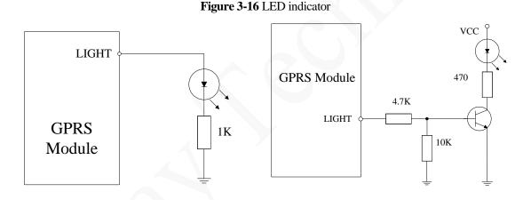
When the module is running, the LED indicator is driven by the LIGHT to indicate different module status with its various blink behaviors. You can set the blink mode by AT commands. For more details, see *Neo\_M590E V1 GPRS Module AT Command Set*.
