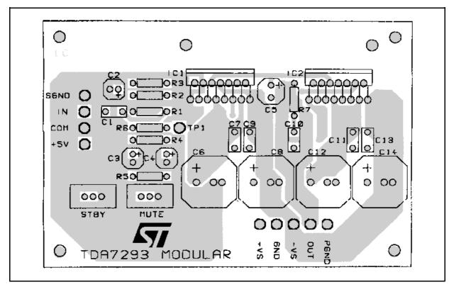
Figure 8a: Modular Application P.C. Board and Component Layout (scale 1:1) (Component SIDE)
