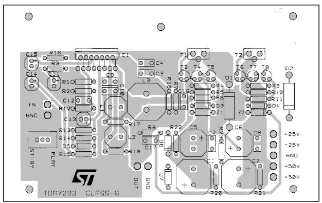
Figure 6b: PCB - Solder Side of the fig. 6.
