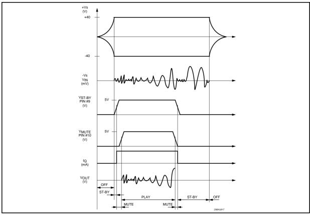
In addition to the overload protection described above, the device features a thermal shutdown circuit which initially puts the device into a muting state (@ Tj = 150 °C) and then into stand-by (@ Tj = 160 °C).
