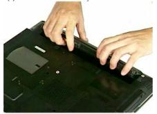
(b) Slide the battery latch to close.
