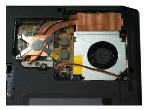
(c).Disconnect the cable on CPU module.
