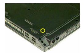
(b) Slide the battery latch to close.
