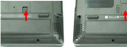
1. Remove Memory cover (a). Remove 2 screws on DDR Door (b) Lift the DDR Door away
