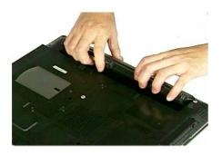
(b). Slide the battery latch to unlock and Firmly slide the other latch to the top and remove the battery
