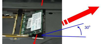
3. If there is an existing memory, remove it by opening the latches (no. 2), which will pop the module up to an angle of 30 degree. Then pull out the memory module in that angle. (no. 3).
