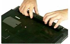
(c) Slide the battery latch to unlock. Firmly slide the other latch to the top and remove the battery.
