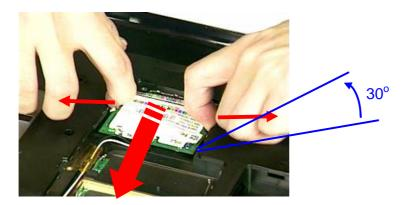
3. Insert new WLAN module at the same an angle of 30 degree, and press down until it clicks into the latches.
