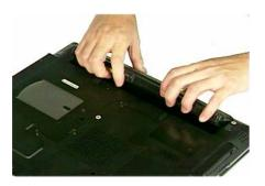
(b) Slide the battery latch to unlock. Firmly slide the other latch to the top and remove the battery.
