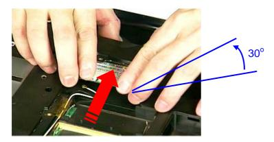
(b). Connect the black cable onto the connector of left side, and the white cable on right side (White cable: AUX, Black cable: MAIN), and then paste 1 pcs of tape to fix the cable.
