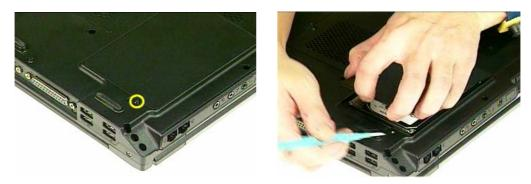
(b). Pull out the hard drive and lift the hard drive away by 2 hands.
