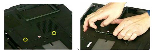
(b). Open the 2 latches aside, which will pop the memory module up to an angle of 30°, then pull out the memory module in that angle
