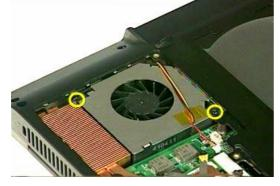
(e).Lift the CPU FAN module away.
