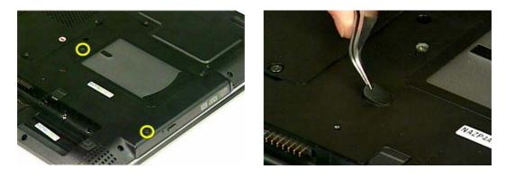
(b). Put the screwdriver (No. 3) here and push the ODD drive out from the NB.
