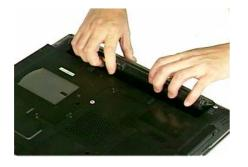
Slide the battery latch (No.1) to close.
